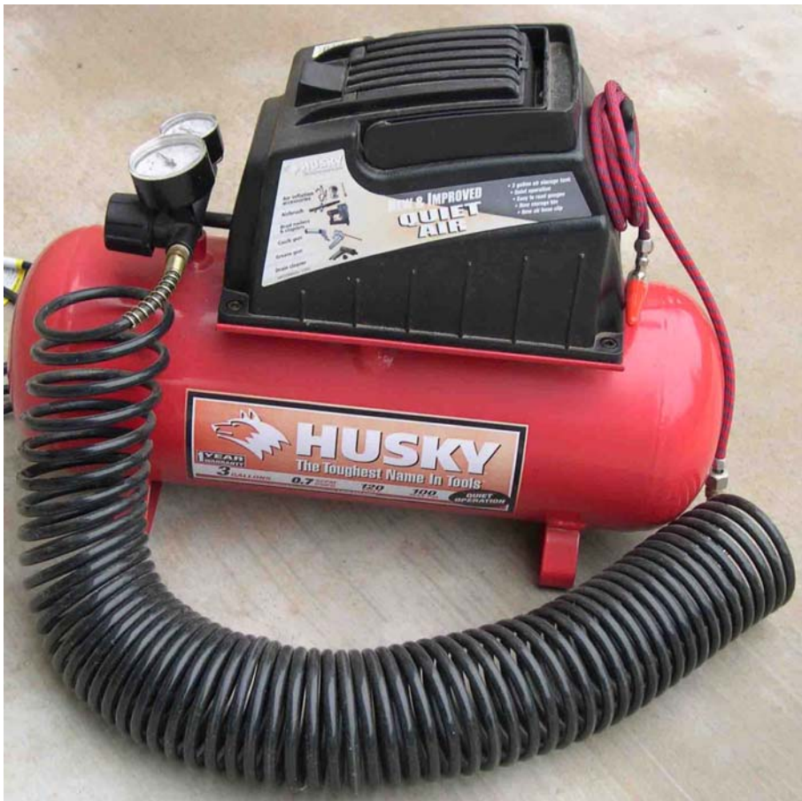
Above: A Workshop Compressor. Motor housed in black box sits on top of red metal air tank. Note the Pressure Gauge and Regulator (round dials on left side). Being
